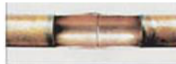
Nitrogen blow performed (No oxidation scale)
